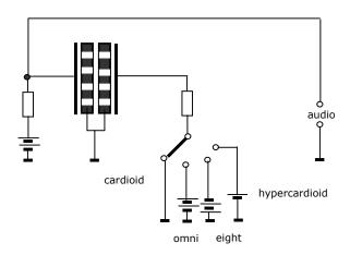
This diagram shows a simplified schematics of the CK12 in the C426.
