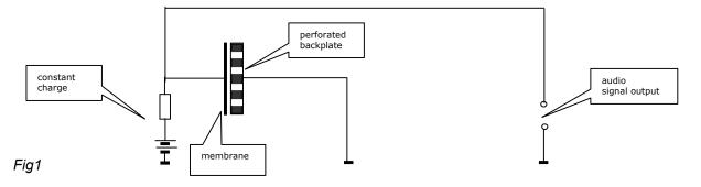
Second we have to consider the directivity characteristics of a microphone. Imagine a capsule as described above with a sealed box (volume) attached to the backplate.
